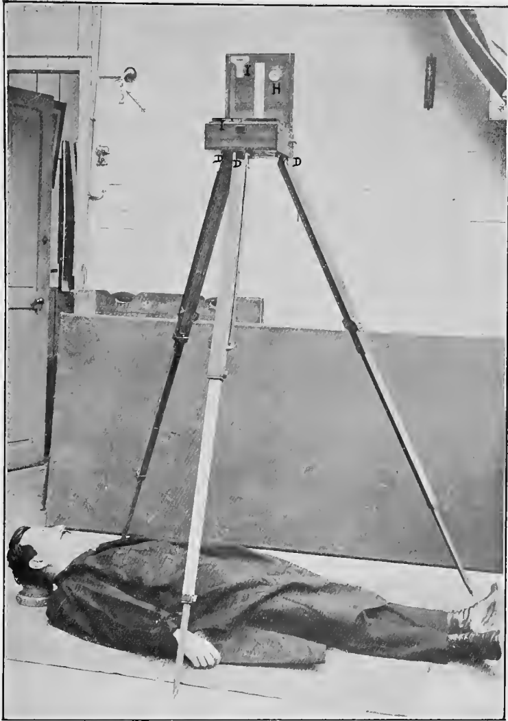
FIG. 2. — The same apparatus in an inverse position for photographing corpses and the ground (traces of foot-steps, spots of blood, etc).
